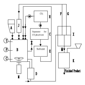
Figure 1 Cycle theory of GAS method for producing toner
